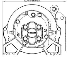
Fig.6 pressure roller, view from bottom
