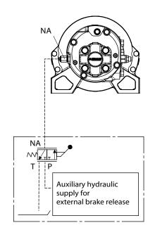
Fig. 11 auxiliary hydraulic supply for external brake release
