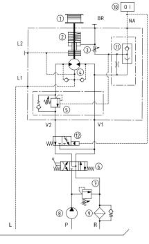
Fig. 10 hydraulic diagram for external brake release
