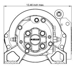
Fig.9 dimensions with pressure roller and rope end switch
